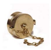
2.5" (65mm) threaded cast brass male plug & chain for protection of female threads used on fire department inlet connections. Also, prevents entry of foreign material. Specify regional hose thread.
