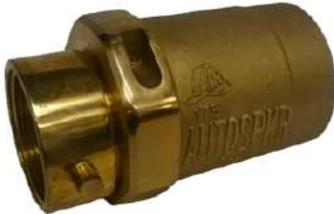
3" (76mm) Female NPT x 2.5" (64mm) Female swivel hose thread, polished brass Check Snoot. The HF325F is used on multiple inlet fire department connections, enabling the connection of several fire department supply lines at one time. The HF325F is equipped with a brass clapper preventing the backflow of water through unused connections. A breakable cap or plug should be installed to protect swivels, and reduce the risk of foreign debris from entering the connection. UL/ULC Listed.
